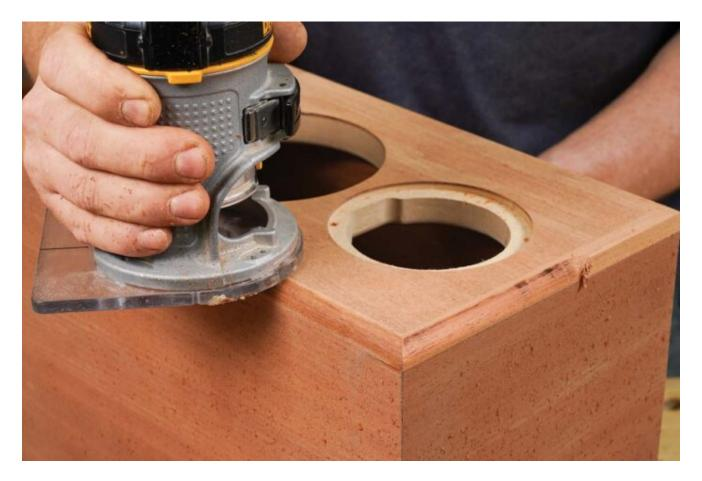
After the glue dries, plane and/or sand the strips flush, and use a 3/8-in. roundover bit to round them.
