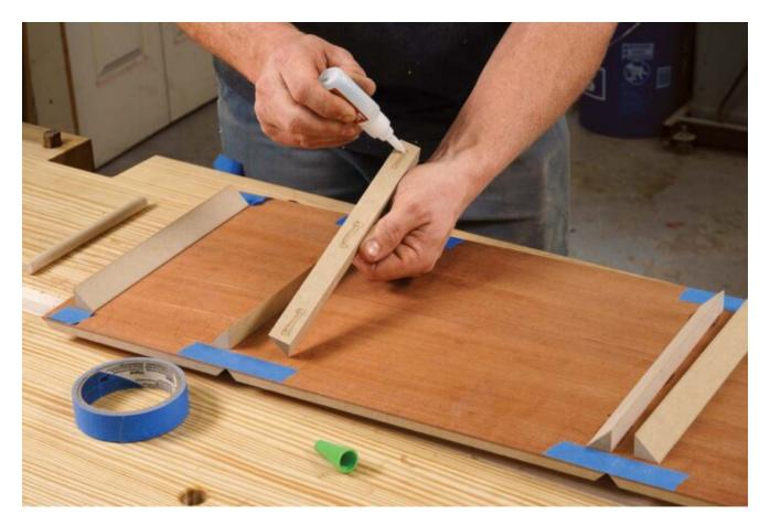
After stretching blue tape across the joints, Gibson uses CA glue to attach 45° MDF blocks. Hold each one in place for 15 seconds before moving on.
