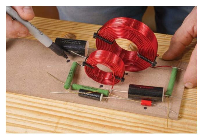
Cut a piece of 1/4-in. MDF narrow enough to fit into the large driver hole, and read the X-Bravo instructions to understand how the parts should be arranged and connected. Position the parts as tightly as possible, and mark and drill holes for zip ties.
