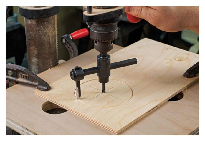
**Make a template for the driver holes.** Drivers need large holes, sometimes rabbeted. Use a circle cutter in the drill press to make templates, factoring in the offset between the router bit and the guide bushing you'll be using.
