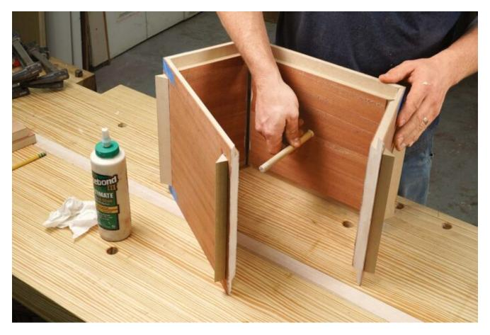
To stiffen the box, the X-Bravo design includes a dowel that connects one side to the other. Drill for this dowel ahead of time, and insert it during assembly.
