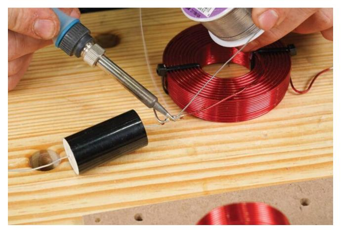
Twist the wires as shown, add flux, and solder the joints. The solder should flow along the entire joint. Check the opposite page for more soldering advice.
