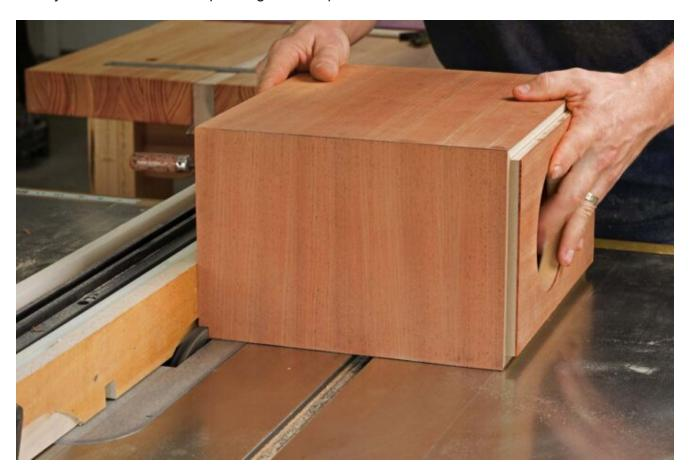
After assembly, the front and back edges get a 3/8-in.-sq. rabbet for solid corner strips.
