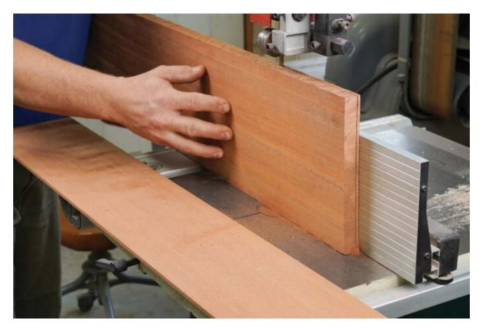
Use a fresh blade, at least 3/8 in. wide, with three or fewer teeth per inch, and center it on the upper wheel. Saw the veneers a little over 1/8 in. thick.
