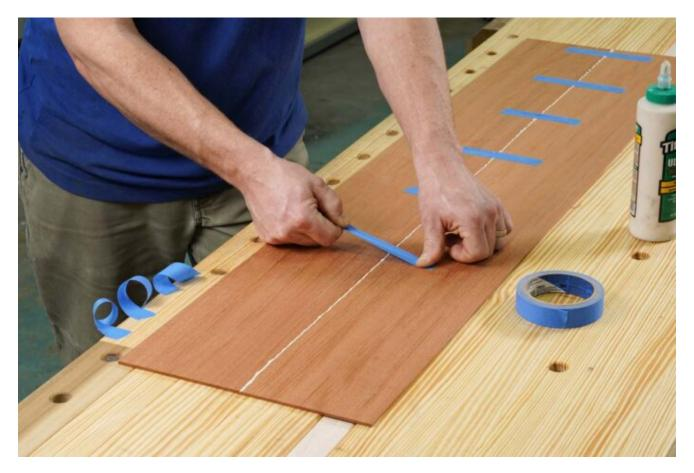
To create wider veneers, join strips. Stretch blue tape across one side of the joint, fold the joint open, spread glue on the edges, fold the panel flat again, and then stretch tape across the other side.
